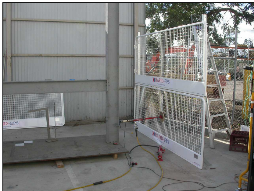
Figure: 4 Subject: Bottom panel outwards horizontal load. .
